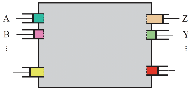
Figure 25.1: Van't Hoff の平衡箱
