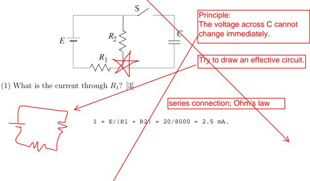
(2) Now, at t = 0 switch S is closed. Immediately after the switch is closed, what are the current  $I_1$  through resistor  $R_1$  and the current  $I_2$  through resistor  $R_2$ ? [4]
