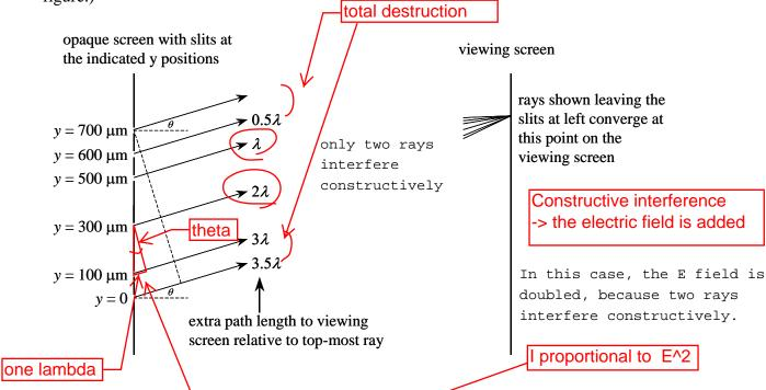
6. The *intensity* of the light measured at the point of convergence of the rays is  $I_6$ . If the intensity of light out of one slit is  $I_1$ , what is the ratio of the intensities  $I_6 / I_1$ ?
