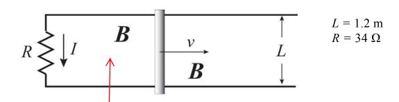
3) The conducting bar is pulled to the right at a constant speed v = 12 m/s.
