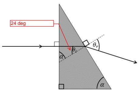
15) A ray of red, monochromatic light travelling in air to the right hits the surface of the prism at 90°, as shown in the figure. What is the angle  $\theta_r$  at which the light emerges?
