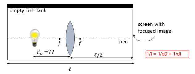
17) Where should a light bulb be placed to produce a focused, real image on the screen inside the fish tank?
