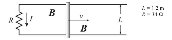
3) The conducting bar is pulled to the right at a constant speed v = 12 m/s.
