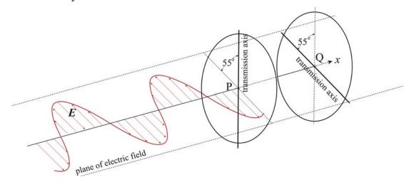
9) What is the amplitude of the electric field  $E_P$  immediately after passing through the first linear polarizer at *P*?
