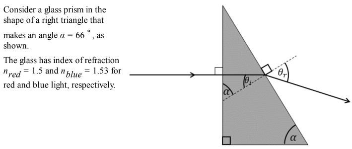
15) A ray of red, monochromatic light travelling in air to the right hits the surface of the prism at 90°, as shown in the figure. What is the angle  $\theta_r$  at which the light emerges?
