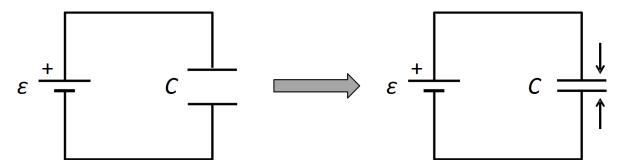
What happens to the charge  $Q \ge 0$  stored on the top capacitor plate? Note that the capacitor remains connected to the battery throughout.
