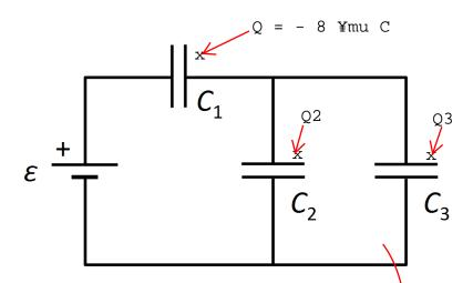
5) How much energy is stored on capacitor  $C_1$ ?
