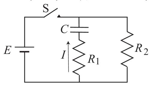
11) Switch S has been closed for a long time. What is the current I through  $R_I$  immediately after S is opened? Pay attention to the direction of the current arrow in the figure.
