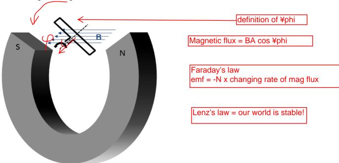
A coil of wire turns between the poles of a permanent magnet as shown in the diagram. The coil has N=34 turns of wire. The magnet produces a constant field of magnitude B=0.119~T. The coil has a cross-sectional area  $A=0.0411~m^2$ .
