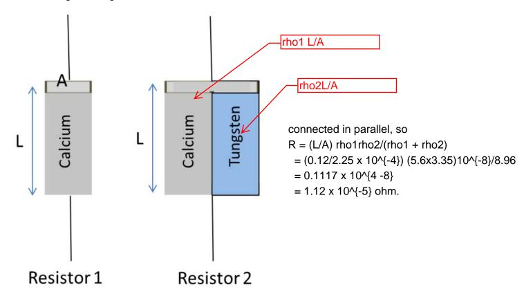
A student decides to build some resistors using rectangular blocks of calcium ( $\rho$  =3.36 × 10<sup>-8</sup>  $\Omega$  m) and tungsten ( $\rho$  =5.6 × 10<sup>-8</sup>  $\Omega$  m). The dimensions of the blocks are identical with a length L = 0.12 m, and cross section A = 2.25 × 10<sup>-4</sup> m<sup>2</sup>. Resistor 1 is created from a single block of calcium. Resistor 2 is created by attaching a block of calcium to a block of tungston as shown in the figure above.
