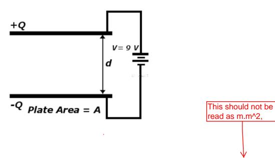
A parallel plate capacitor consists of two metal plates with an area  $A = 542 \text{ mm}^2$  separated by a distance d = 0.36 mm. The capacitor is connected to a 9 volt battery as shown above.
