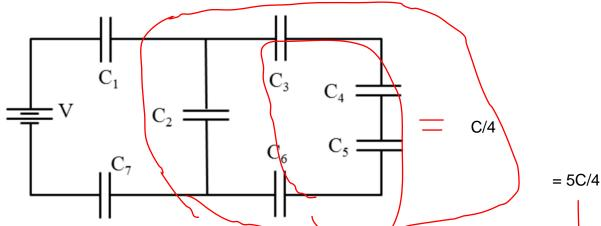
Seven identical capacitors with capacitance C = 8.5 nF are connected to a 12 Volt battery as shown in the figure above.
