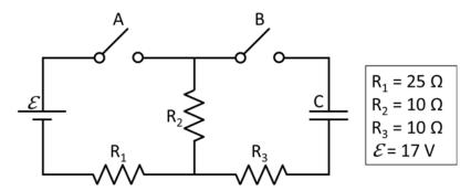
At time t=0 switch B is closed (switch A remains open).
