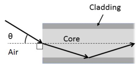
17) What must be the maximum incident angle  $\theta$  of the beam at the air-core interface, as shown in the figure, such that light cannot escape through the cladding of the optical fiber?
