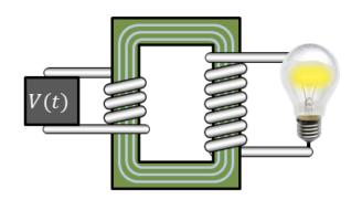
6) What is the maximum number of turns on the secondary coil for the output voltage not to exceed 115 V when the voltage on the primary coil is V = 20 V?
