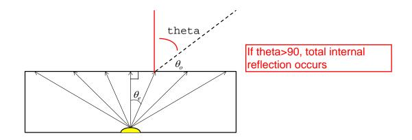
16. What is the maximum emission angle  $\theta_{e,max}$  for which light is observed above the surface (the pool is as wide as it needs to be)?
