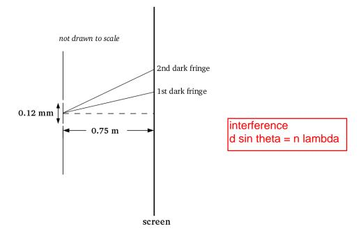
25. What is the distance,  $y_2 - y_1$ , between the first and second dark fringes located from the central axis? Assume the distance between the fringes on the screen is much smaller than the slit-to-screen distance (that is,  $y_2 - y_1 << 0.75$  m).
