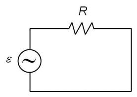
You measure the *rms* (root mean square) current,  $I_{rms}$ , flowing through the resistor using an ammeter and obtain  $I_{rms} = 3.57$  A. What is the maximum generator voltage,  $\varepsilon_{max}$ ?
