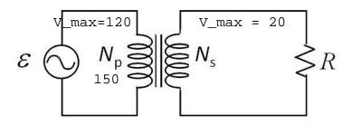
23. Find  $N_s$  for which the maximum induced voltage in the secondary coil is 20 V.
