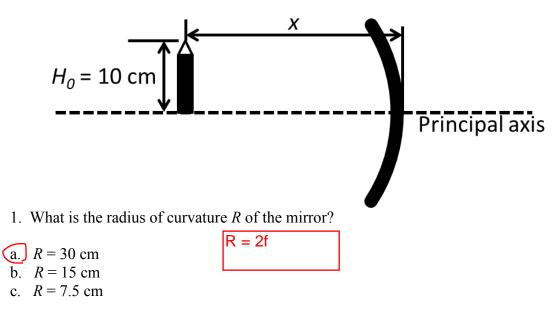
2. At what position x in front of the mirror should the pencil be placed such that its image appears to be 60 cm <u>behind</u> the mirror? 1/f = 1/do + 1/di
