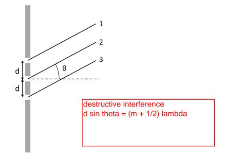
At the angle shown, rays 1 and 3 interfere destructively. Each ray has intensity  $I_0$ .
