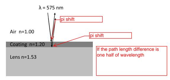
20. The coating works in such a way that yellow light of wavelength  $\lambda = 575$  nm (in vacuum) is <u>NOT reflected</u>. Which of the following is a possible value for the coating thickness *t*? wavelength in coating: 575/1.2 = 479.17 nm
