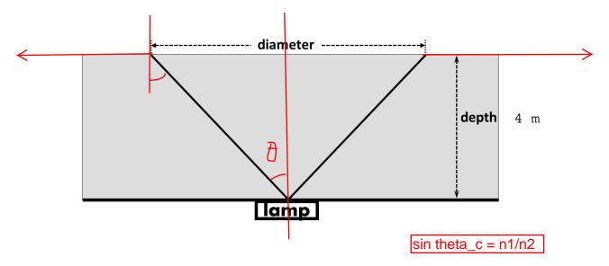
What is the diameter of the circle of blue light  $D_{blue}$  from this lamp observed on the surface of the pool (as indicated in the figure)?
