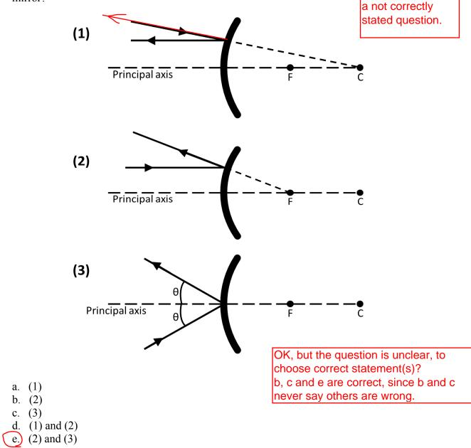
5. Which of the following figures <u>correctly</u> represents a ray reflected off a convex mirror?
