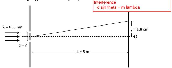
18. If the second order bright fringe is at a position y = 1.8 cm on the screen, what is the separation  $\overline{d}$  between the two slits?
