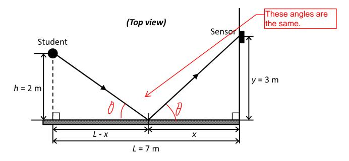
At what distance *x* away from the wall must the incident beam hit the mirror?
