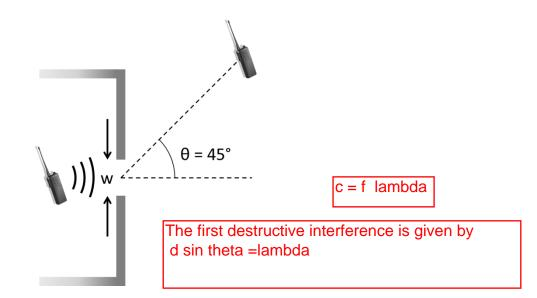
24. You notice that if you stand outside at an angle of  $45^{\circ}$  relative to the doorway, you DO NOT receive your friend's radio signal because of destructive interference. What is the frequency *f* of the radio wave?
