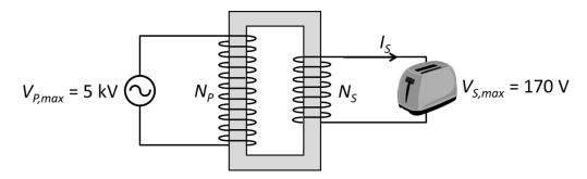
16. What is the ratio  $N_P/N_S$  between the number of turns in the primary  $(N_P)$  and the number of turns in the secondary  $(N_S)$ ?
