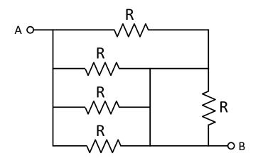
17. In the network of resistors above, the 5 resistors have the *same* resistance R. Calculate the equivalent resistance between points A and B in terms of R.
