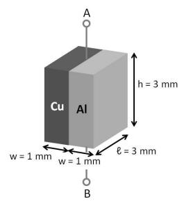
19. Suppose wires are attached to the top and bottom surfaces of the resistor, at positions A and B. What is the resistance measured across A and B?
