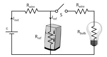
13. Let  $I_{out,open}$  be the current out of the outlet when the light switch S is open (i.e when the light is off). Now the light switch S is closed, turning on the light. The current  $I_{out,closed}$  out of the wall outlet
