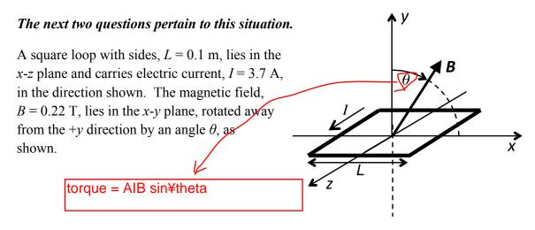
26. What value of  $\theta$  would make the torque on the loop equal to zero?
