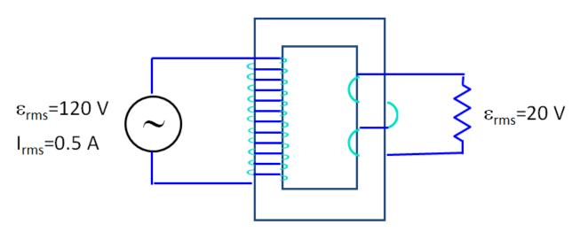
3. What is the rms current on the secondary side of the transformer?
