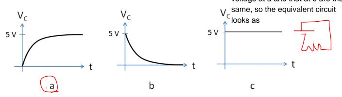
a. a After a long time, C is charged up to 5V.
