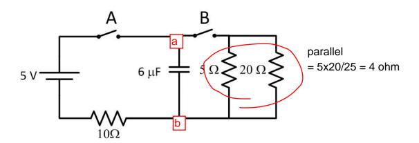
5. Switch A is closed at time t=0 and switch B is left open. Which graph shown below best represents how the <u>voltage  $V_C$ </u> across the capacitor changes with time t? Initially, C is not charged, so voltage at a and that at b are the
