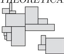
Figure 29.3: Fundamental set: it is a figure made of a finite number of rectangles whose edges are parallel to a certain Cartesian coordinate axes and the rectangles do not overlap except at edges and vertices. Its area is the total sum of the areas of the constituent rectangles.
